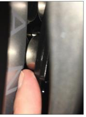
With the bolts only loose enough to shift the magnets side-to-side, adjust them so you feel an even spacing between the magnets and the disc.
